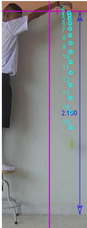
(a) Chute libre. Tiré de *Digital video analysis of falling objects in air and liquid using Tracker*, Siri-sathitkul et Al.
